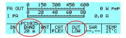
Once the correct preset is adjusted, go to TX mode (RTTY, CW) to verify the output power.
