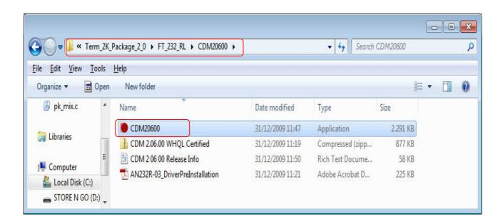
This application has the purpose of properly installing the USB drivers. So, without making any physical link between the EXPERT 2K-FA and the PC, let's double-click, using the mouse left-button, over the "red ball" icon of CDM20600.exe application and wait for its preparatory job completed.
