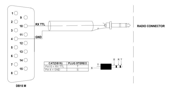
This interface is standard for all the Icom models equipped with CAT. The cable always terminates to a 3.5 mm. mono plug.
