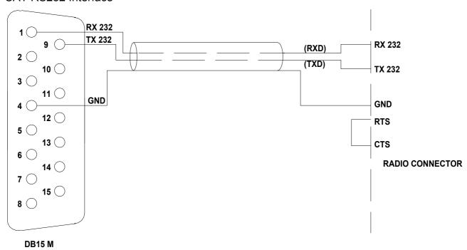
The Radio connector could be DB-9 or DB-25 male connector or female connector (read the specific manual). In the manual, also verify if the RTS-CTS link is necessary.
