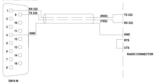
The radio connector may be a DB-9 or DB-25 male connector or female connector (read the specific manual). Verify from the manual if the RTS–CTS link is necessary.
