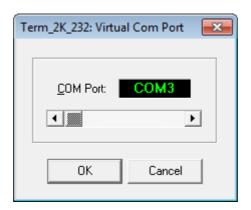
With all the serial resources connected go to Control Panel >>> Hardware and Sound >>> Device Manager and choose a serial COM listed in the HW configuration but not used by other applications.
