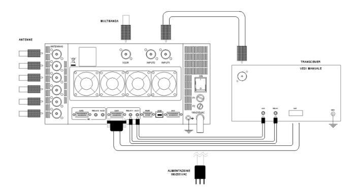
The diagram shows the connections with one transceiver only. To connect the second transceiver repeat the same connections using the port "IN 2".
