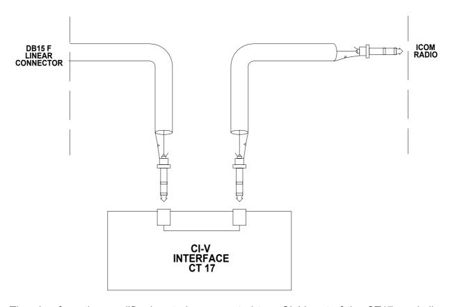
The plug from the amplifier has to be connected to a CI–V port of the CT17 or similar device. The transceiver has to be connected to another CI–V port.
