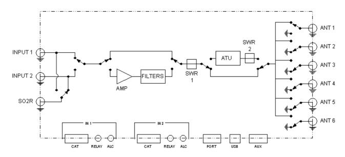
The position of the contacts, as shown in the diagram, is the situation of the linear amplifier in OFF state.
