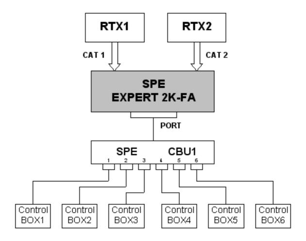
In this case you need to connect the unit control box outputs 1,2,3,4,5,6 in accordance respectively with the antennas ANT 1,2,3,4,5,6.
