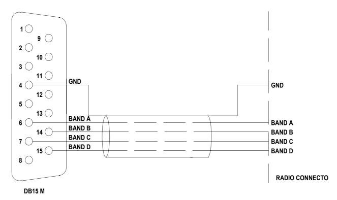
Without the CAT, the band is commanded by four digital signals (Band A, Band B, Band C, Band D). Refer to the specific manual.
