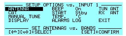
a) ANTENNA An appropriate antenna may be assigned to each band selecting the (ANT 1, ANT 2, ANT 3, ANT 4, ANT 5, ANT 6) connector. If you don't have an antenna for a particular band, input "N".
