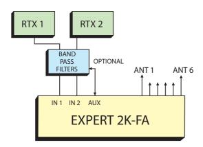
Automatic tuner remotable on the roof (option), you can automatically manage up to 6 antennas with just one coaxial cable feed.
